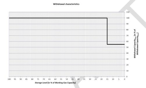
From a Storage Level ≤ 15% the Withdrawal Capacity<sub>firm</sub> is reduced to 55%.
